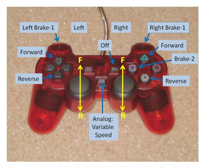
The ANALOG button toggles between digital and analog mode. An LED in the unit will glow dimly when in analog mode.
