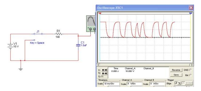
You change the switch position by pressing the space bar on the keyboard. You must have Electronic Workbench window active, not the Oscilloscope window to do this.
