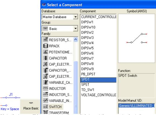
Note that you will have to rotate the switch to get the correct orientation.
