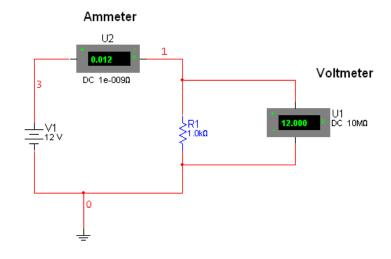
The following shows how to find the components you want for this circuit. On the left is the desired component symbol. Next is the menu icon to click, and on the right is window which opens. The entries which you select are shown greyed. On the first one, the entry "POWER SOURCE" is selected and "DC\_POWER" is selected. On the right is the symbol which will be placed on your workspace.
