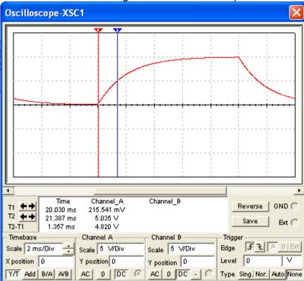
Note on the digital readout the Channel A voltage at T2 is 5.035V. The time it took to reach that value is T2-T1 = 1.357 ms.
