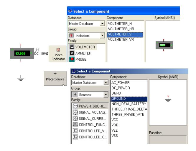
Ohm;s :Law says the current in this circuit should be V/Rv12/1000 = 0.012 amps = 12 milliamps (ma)
