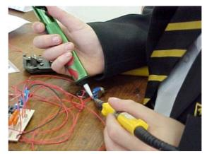
Using a desoldering pump (solder sucker)
