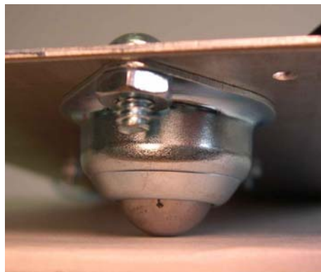
Figure 6: Roller ball mounted to TekBot's frame
