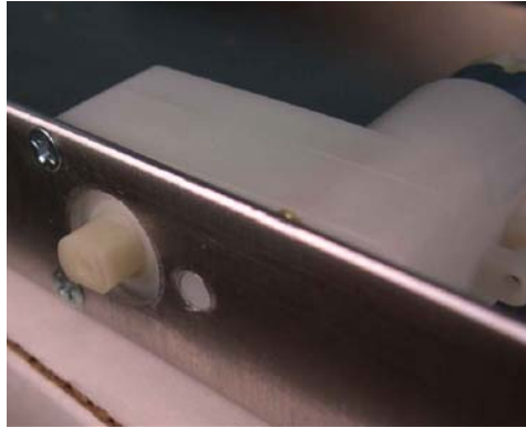
Figure 3: Motor mounted to TekBot frame.
