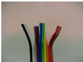
Figure 1: Ribbon cable used to connect motors.
