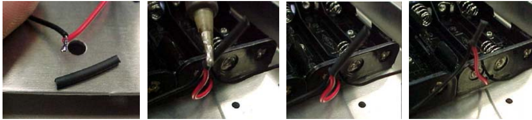
Figure 5: The step for shrink tubing a connection.
