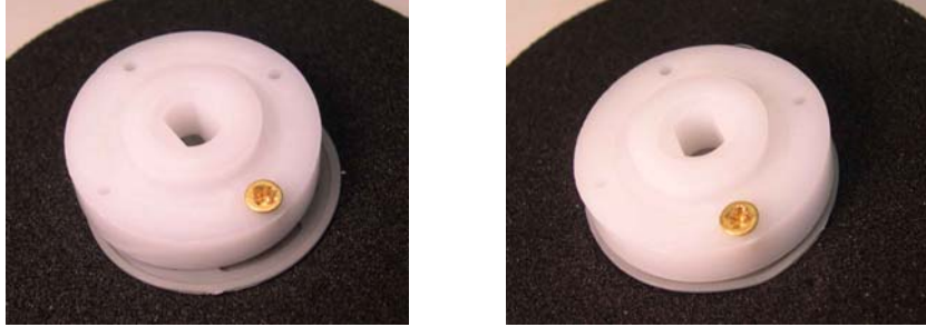
Figure 7: Un-aligned and aligned adapter disk
