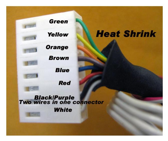
The Black wire and Purple wires are crimped in one connector
